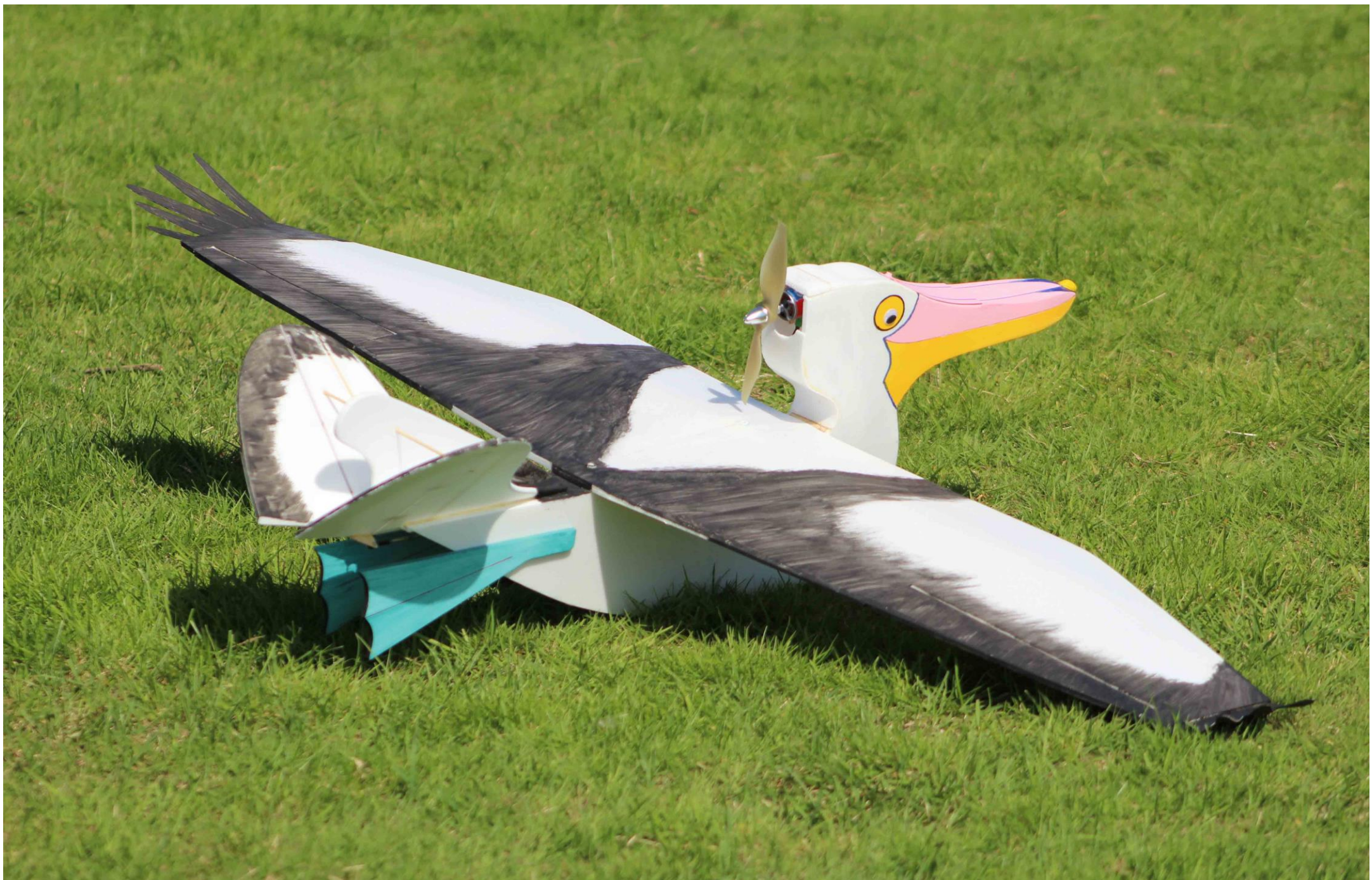
Guy's Pelican is powered by a single electric motor, in the head.
