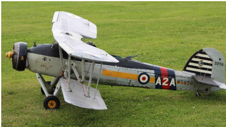
The Fairey Swordfish demonstrates it's scale folding wings, which enabled storage below the deck of aircraft carriers. The Swordfish saw service throughout WW2, and outlived it's planned successor, the Fairey Albacore.
