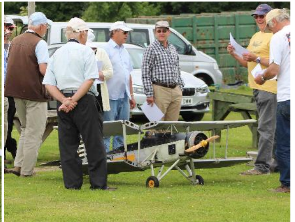
The Fairey Swordfish demonstrates it's scale folding wings, which enabled storage below the deck of aircraft carriers. The Swordfish saw service throughout WW2, and outlived it's planned successor, the Fairey Albacore.
