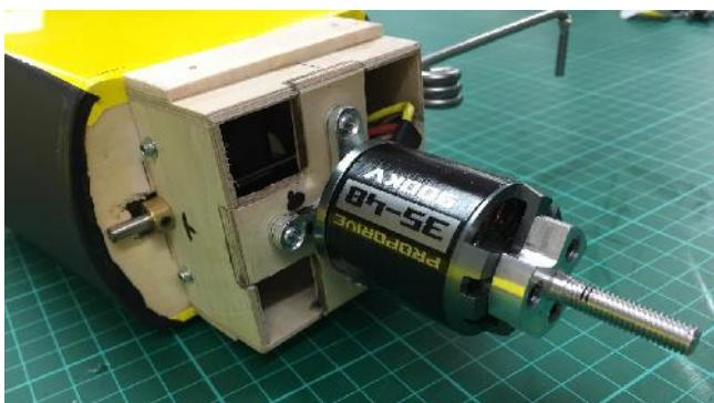
Mounting the motor was not that hard, but Robert reports that he had to modify the cowl to incorporate an air scoop to provide enough of an airflow to cool the motor and speed controller. The motor is a PropDrive 38-45 900Kv motor from Hobbyking, with a 80amp ESC. Power is provided by a 4S 4200mAh Li-Po battery. There is no detail available on where the battery lives – possibly in the tank bay under the hatch?
