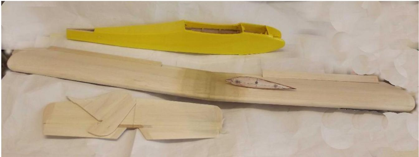
*The new trainer takes shape. The aerofoil shape on top of the wing is the plywood template used to cut the foam wing core from expanded polystyrene insulating foam. A template is pinned to each end of the foam slab, and the wing section is then cut by drawing a thin electrically heated wire across the templates from front to back.*
