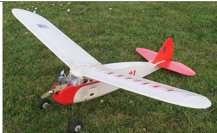
Paul Notley's Utility has been excellently built over the winter from a Ben Buckle plan and is powered by an OS 40 4stroke.
